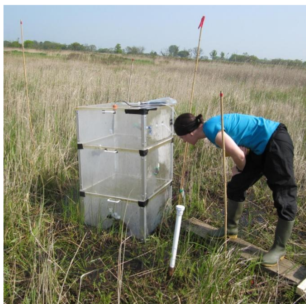
Figure 1.1 Left: Photograph of collar, flux chamber and three flux chamber extensions. This shows a near-final prototype that is very similar, except in details like the handles, to those that were used across the project. Right: the prototype being used at the NB-LN site.
