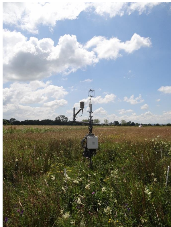
Figure 2.1: Eddy covariance instrumentation at the Tadham Moor (SL-EG) site in Somerset. The left panel shows an R3-50 sonic anemometer (Gill Instruments Ltd, Lymington, UK) and A LI7500 infrared H 2 O/CO 2 analyser (LI-COR Biosciences Ltd., Lincoln, Nebraska, USA). The right panel shows the eddy covariance system installed over the vegetated canopy on 11 th July 2014 (photographs: R. Morrison, Centre for Ecology and Hydrology).
