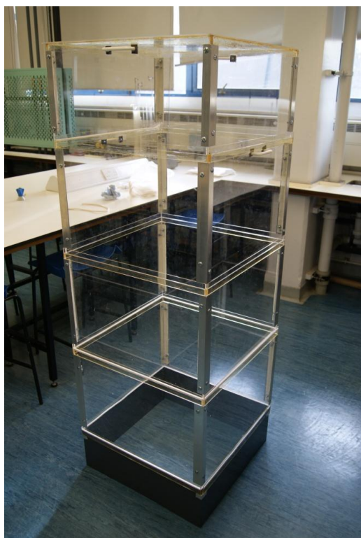
Figure 1.1 Left: Photograph of collar, flux chamber and three flux chamber extensions. This shows a near-final prototype that is very similar, except in details like the handles, to those that were used across the project. Right: the prototype being used at the NB-LN site.
