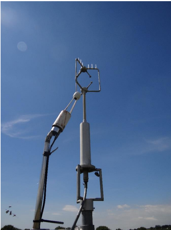
Figure 2.1: Eddy covariance instrumentation at the Tadham Moor (SL-EG) site in Somerset. The left panel shows an R3-50 sonic anemometer (Gill Instruments Ltd, Lymington, UK) and A LI7500 infrared H 2 O/CO 2 analyser (LI-COR Biosciences Ltd., Lincoln, Nebraska, USA). The right panel shows the eddy covariance system installed over the vegetated canopy on 11 th July 2014 (photographs: R. Morrison, Centre for Ecology and Hydrology).
