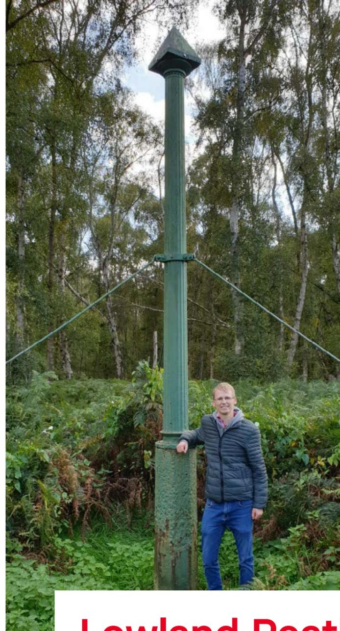
Figure 1: The Holme Post at Holme Fen, Cambridgeshire. In 1851, a metal post was driven into the peat so that its top was level with the ground. The top of the post is now 4 m above the land surface. At 3 m below sea level, Holme Fen is the lowest point in Britain. (Photo – S. Page).
