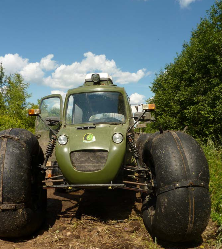
Figure 4 Biomass harvester with balloon tyres to improve trafficability on wet peat soils (Photo: J. Clough)
